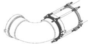
Restrain movement of pipe in the fitting bell, when concrete thrust blocks are impractical. Includes clamps, assembly nuts and bolts and eye bolts that connect to bell (shown on bell).
